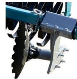
Double spring protection STANDARD
